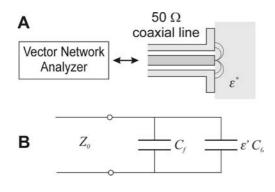
Fig. 4. A - Open-ended coaxial probe in the form of coaxial line open to the space with material of unknown dielectric permittivity  $\varepsilon^*$ , B - modelling the discontinuity of electromagnetic field by lumped capacitances  $C_f$  and  $C_0$ .
