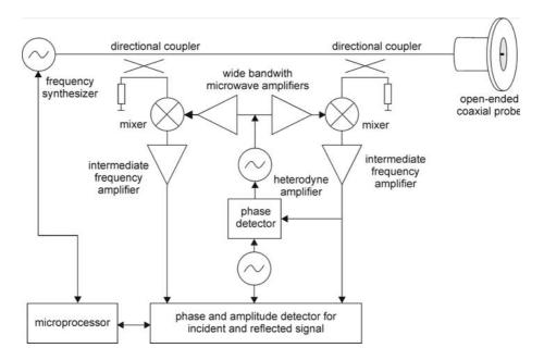
Fig. 3. Basic elements of the frequency domain reflectometer for determination of complex dielectric permittivity of porous media.
