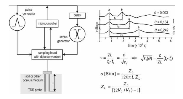
Fig. 2. Basic elements of the time domain reflectometer for determination of velocity of propagation of electromagnetic waves in porous media.
