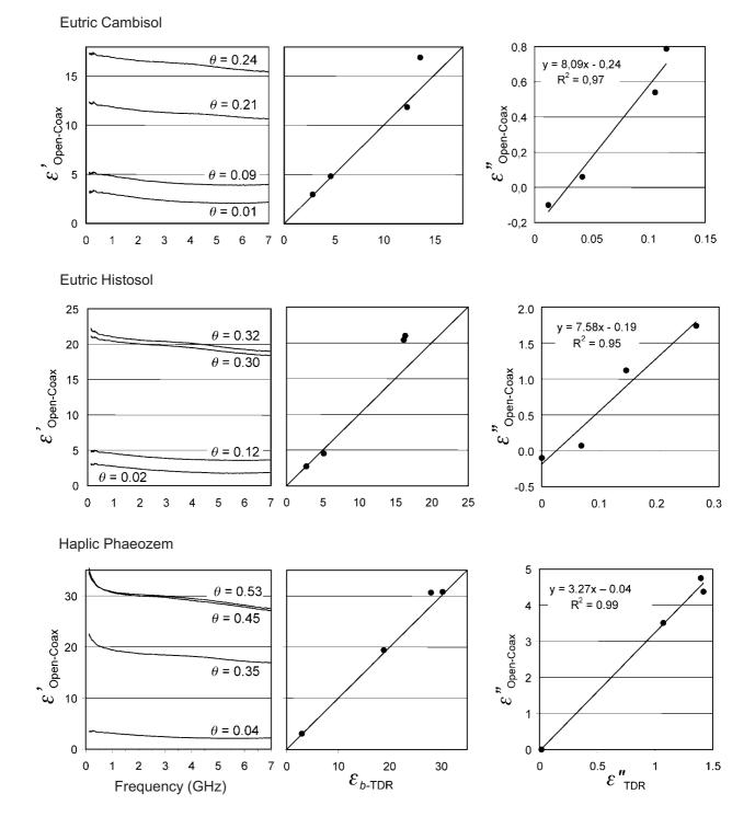
**Fig. 7.** Comparison of real,  $\varepsilon$ ', and imaginary,  $\varepsilon$ ", parts of the complex dielectric permittivity for the selected soils, calculated from the TDR and Open-Ended Coax probe measurements;  $\varepsilon_{b-TDR}$  is the bulk dielectric constant measured by TDR.
